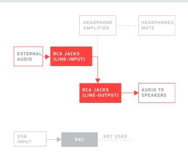
Element's RCA outputs are true Line Outputs. The Headphone Amplifier's knob adjusts the headphone output. DAC line-level output may be adjusted at your PC, or at your receiving amplifier or speakers.
