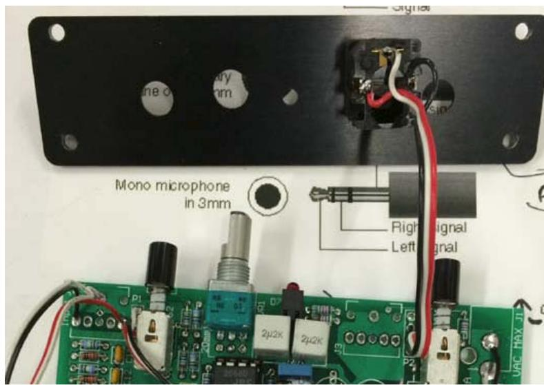
Attach headphone jack to front plate after completing all other assembly. Black nut is secured by a compression fit. With jack & nut installed on front plate, use table surface to apply pressure to nut. After nut snaps in place, gently rotate 1/4 turn clockwise.
